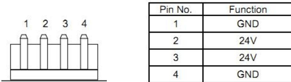
Figure 2-7 Power socket and pin assignment
